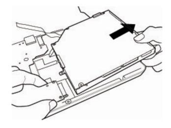
Figure 4-28 Removing ODD
